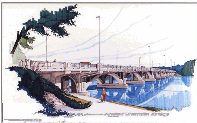
Fig. 7-9. Rendering of historic structure to be widened, historic integrity of original construction preserved, Anoka/Champlin Bridge, Minnesota
