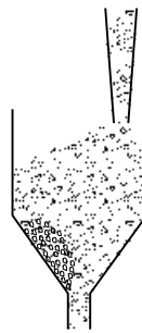
INCORRECT Dropping of concrete on sloping sides of bucket.
