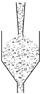
CORRECT Dropping of concrete directly over gate opening.
