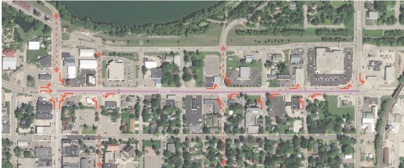
Figure 8. Bicycle Movements with a High Number of Red Bicycle Design Safety Flags
