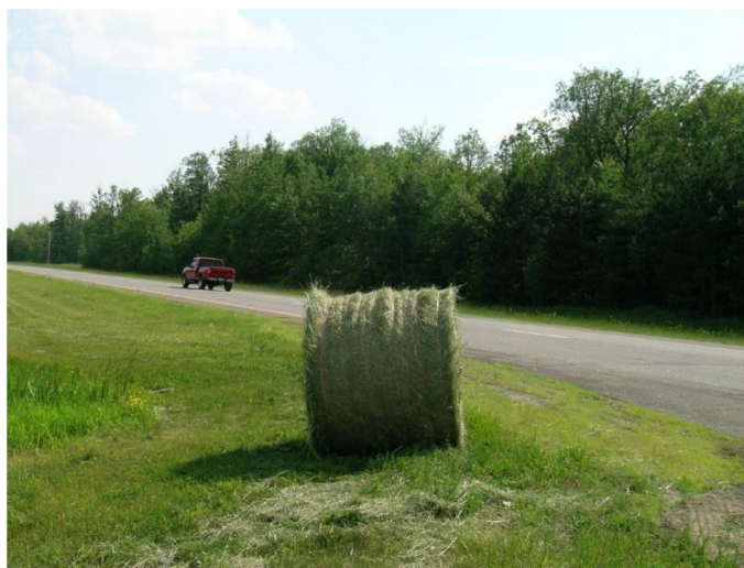
FIGURE 20: A HAY BALE ON THE ROADSIDE. IMPROPERLY LEFT IN THE CLEAR ZONE
