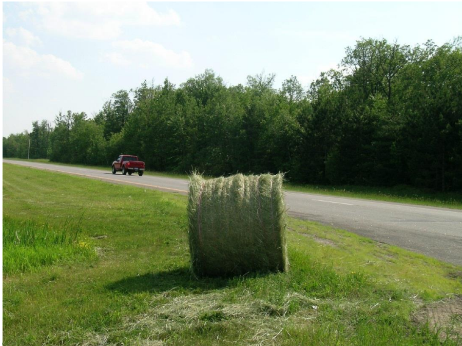
FIGURE 20: A HAY BALE ON THE ROADSIDE, IMPROPERLY LEFT IN THE CLEAR ZONE
