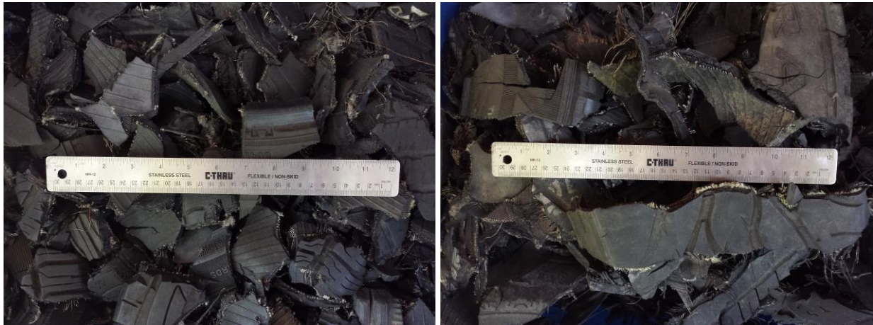
Figure 1-2: Left - Type A TDA, Right - Type B TDA
