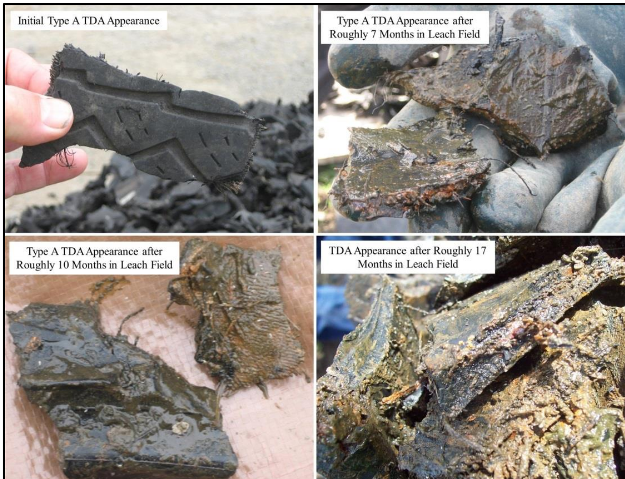
Figure 3-2: Microorganism Growth on TDA after 7, 10, and 17 Months of Wastewater Loading In Leach Fields (Finney et al. 2013)
