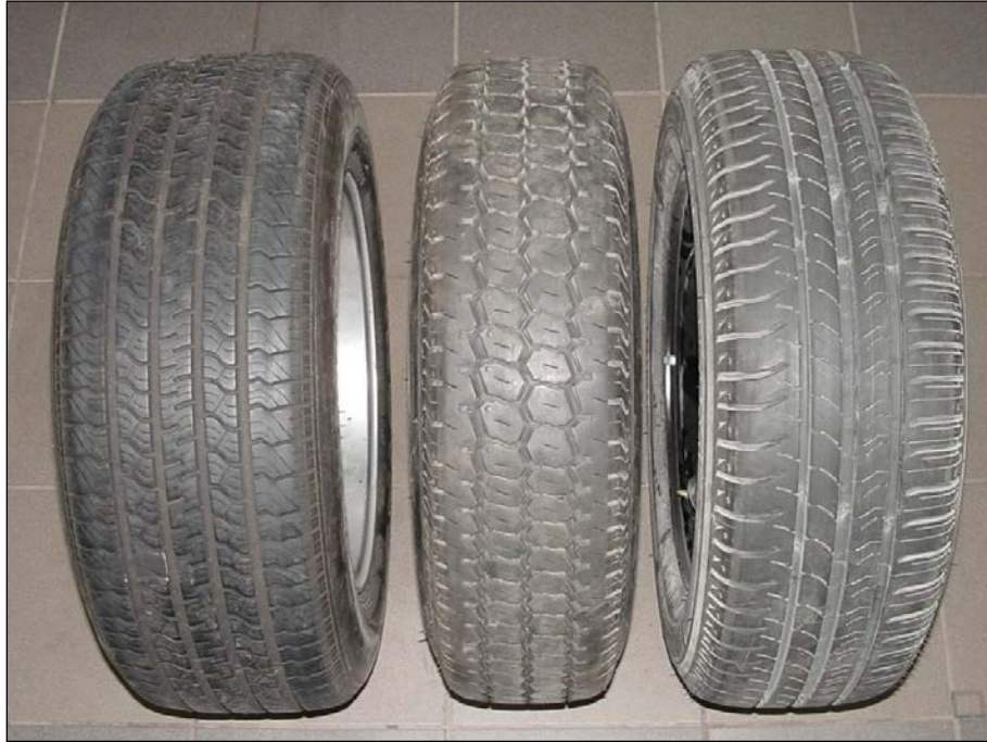
Figure 2-1. Test tires used in the rolling resistance testing at MnROAD.
