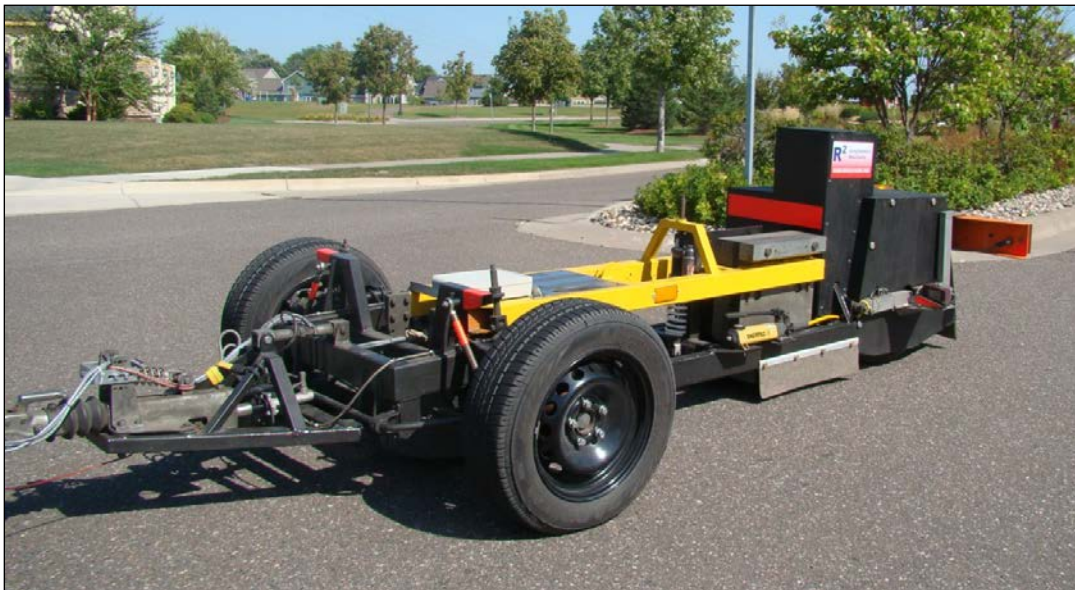
Figure 1-1. Rolling resistance test trailer.
