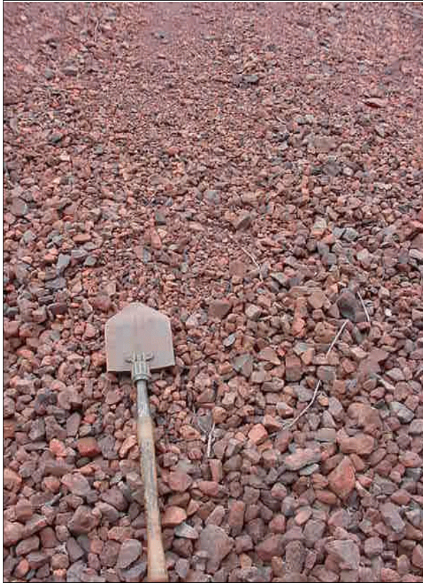
Figure 7. Picture of coarse tailings. Note the range of material size. Shovel is 2 feet long.
