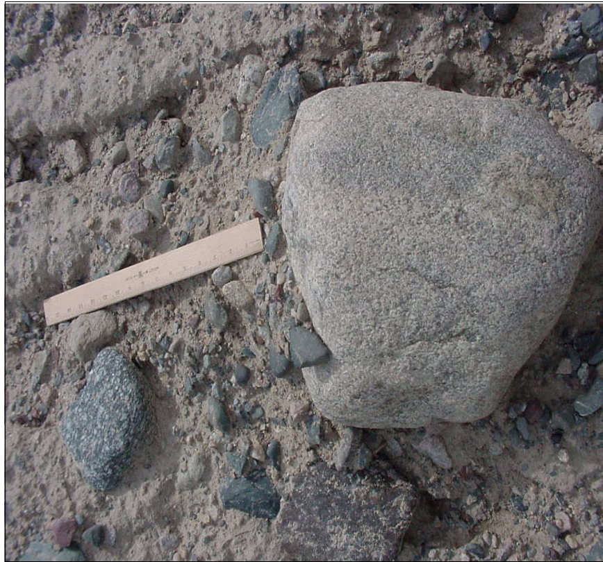
Figure 5. Picture of glacial till. Note the grain size ranges from silts to boulders. Twelve inch ruler is for scale.
