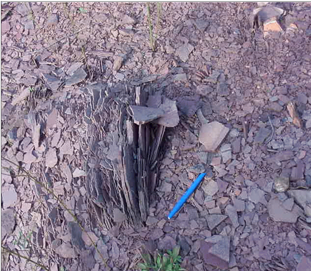
Figure 6. Picture of material called slate. Fractures occur along bedding planes. Pen is for scale.
