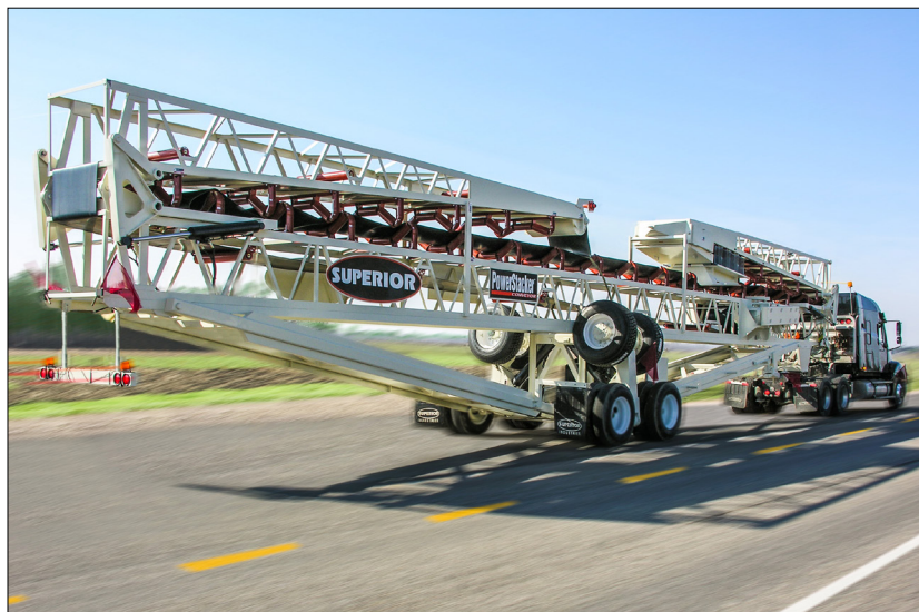
Superior Industries builds conveyor equipment such as the Powerstacker, a stacking conveyor, seen above.
