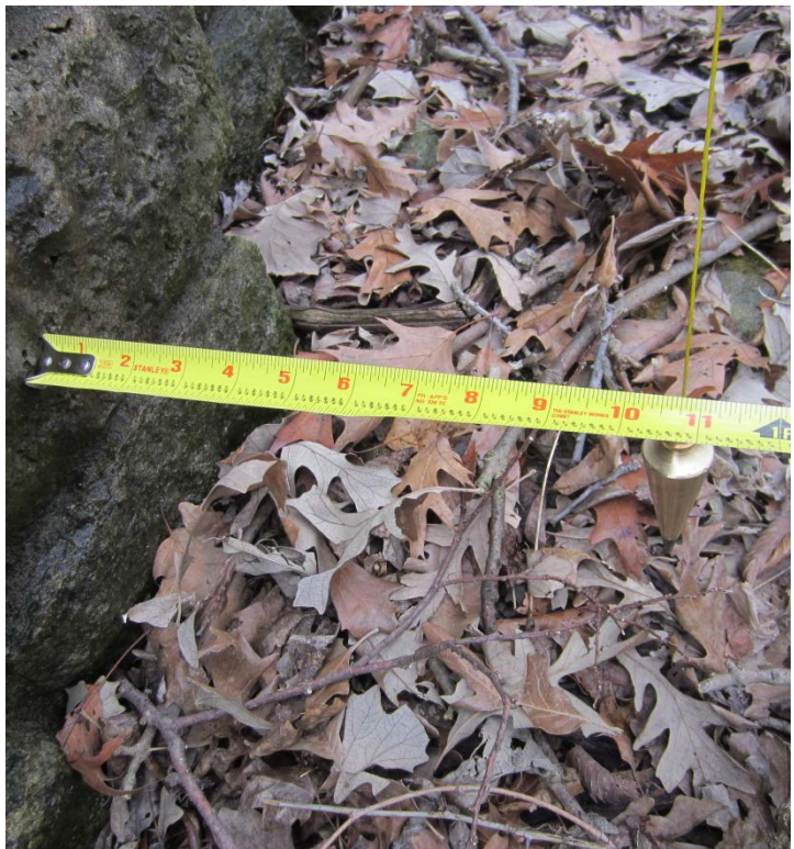
4.6 – West end of North Overlook Wall is out of plumb by 9-1/4" (above left) at the west pier is and the east pier is out of plumb by 10-3/4" (above right)
